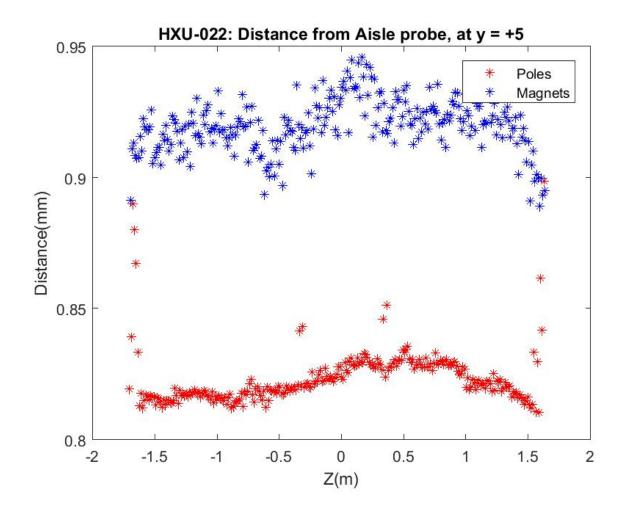
Probe2 Capacitive Sensor Readings y = +5mm
