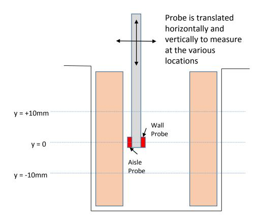
The following plots show the pole and magnet position measurements. The ANL system has two back-to-back capacitive probes on one probe holder. The x and y stages on the bench are positioned so that the probe is in the proper location for each of the 6 scan locations.
