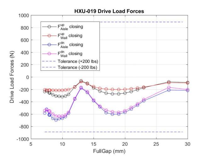
The Forces were only recorded as the gap was closing, and for the gaps that were measured with the Hall Probe.
