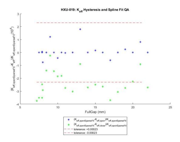
Plotted functions have been calculated from measured values open Keff (opengap) and closeKeff (closegap) using the following Matlab calculations:
