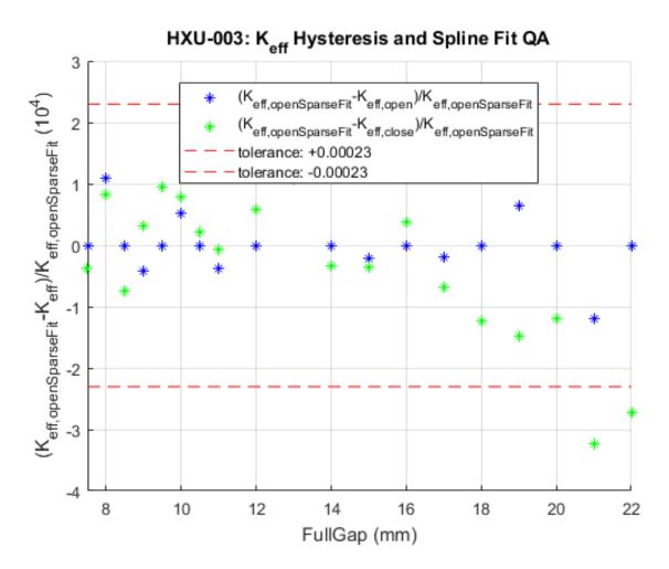
Plotted functions have been calculated from measured values openKeff (opengap) and closeKeff (closegap) using the following Matlab calculations:
