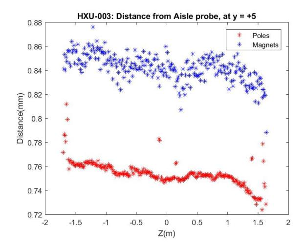
Probe2 Capacitive Sensor Readings y = +5mm
