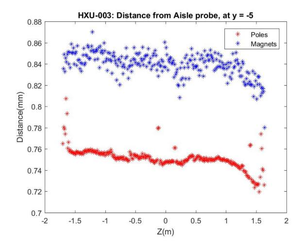
Probe2 Capacitive Sensor Readings y = -5mm
