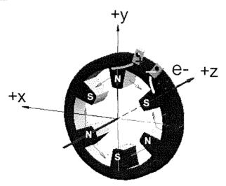
Determine the electrical connection polarity (with supply outputting positive current) which produces the required magnetic field polarities.
