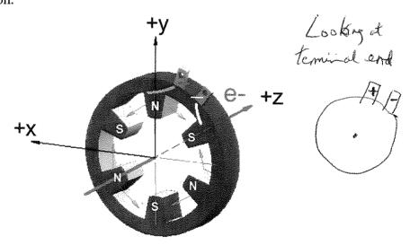
Determine the electrical connection polarity (with supply outputting positive current) which produces the required magnetic field polarities.
