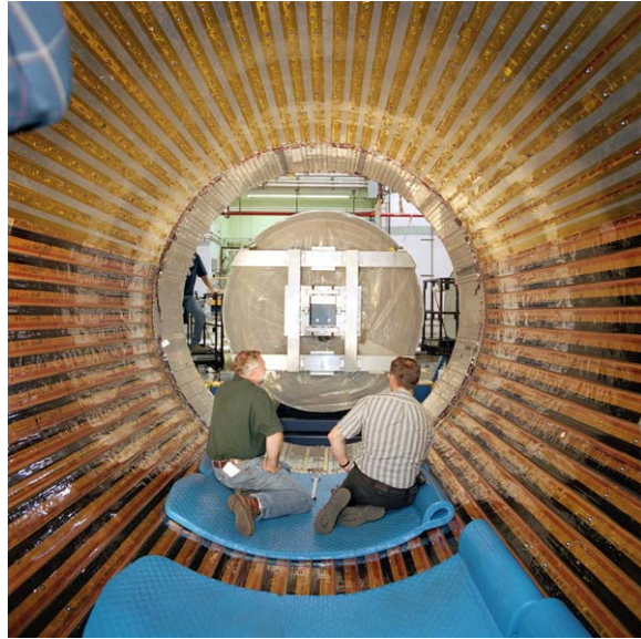
Figure 18 – COT insertion with TOF on solenoid bore
