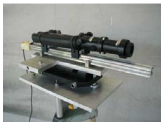
Figure 3 : the electronic "mole" and the laser
