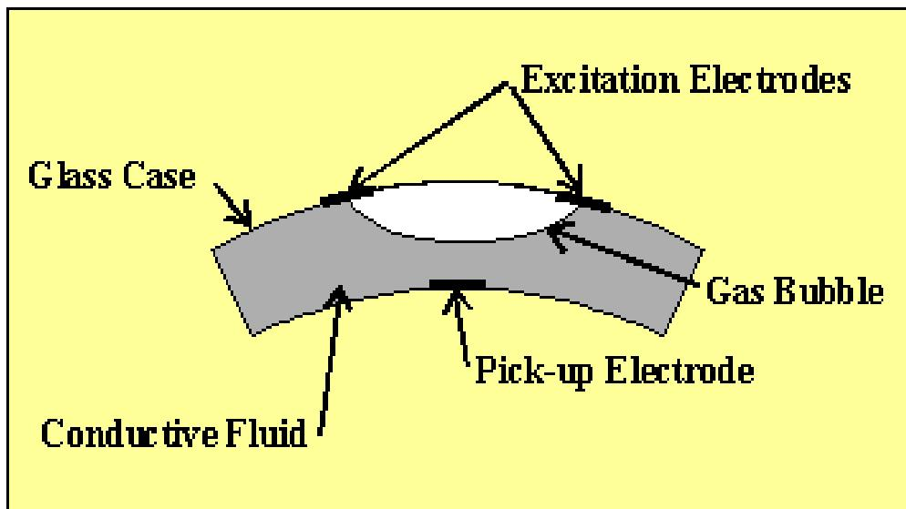
Fig.4 Principle of electrolytic tilt sensor operation
