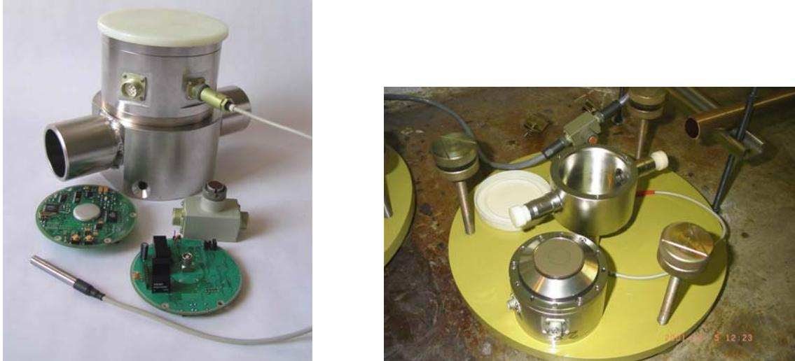
Fig.12 Partly disassembled SAS monitors
