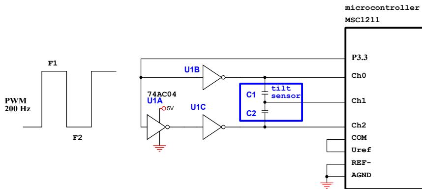
Fig.5 Circuit diagram of tilt measurement principle
