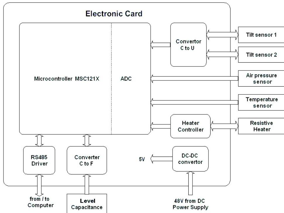
Fig.6 Functional circuit diagram of SAS electronics
