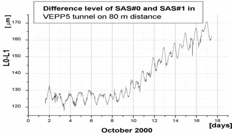
Fig.10 SAS measurement example of ground motion
