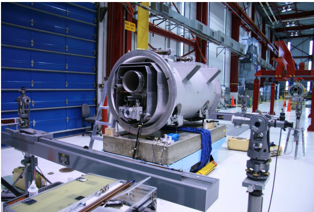
Figure 12: Dual alignment telescopes setup
