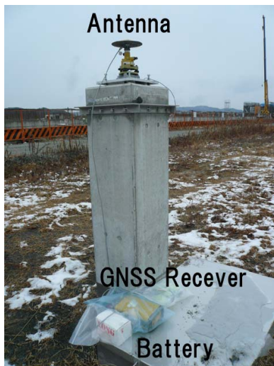
Fig. 12. GNSS system around the monument.
