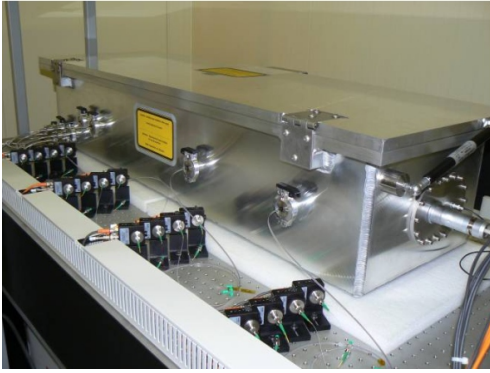
Figure 4: An evacuated chamber contains the Reference Interferometry System, which is read-out by fibre-ribbons routed through custom vacuum feedthroughs to an external array of photodiodes.
