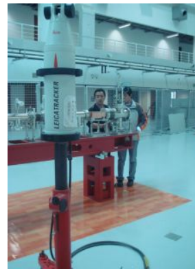
Figure.8: Pre-alignment of ID front-end
