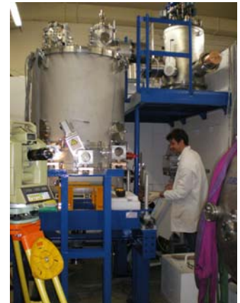
Figure 14: Measurement of cavity displacements, IPN-Orsay,
