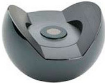
Figure 6: Special target for photogrammetric measurements, which can be replaced by laser tracker targets, using the respective sphere mounts.
