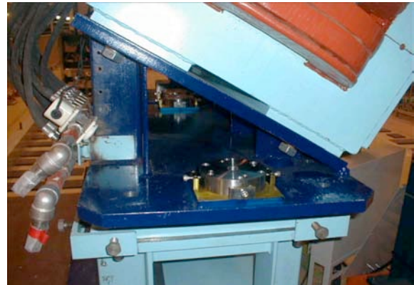
Figure 4: Additional magnet stand to create large rotation angles, around and along the beam directions. Two new reference plates were added on the magnet support.
