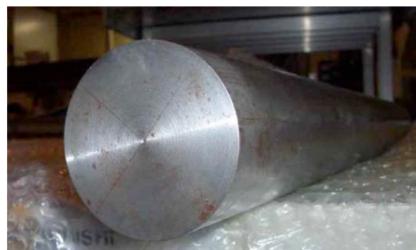
Figure 12: An iron rod for Q1/Q2 alignment. The rod center is marked to be viewed by the transit.
