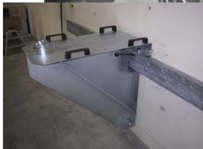
Moveable bracket on track with tilt adapter to increase vertical working range
