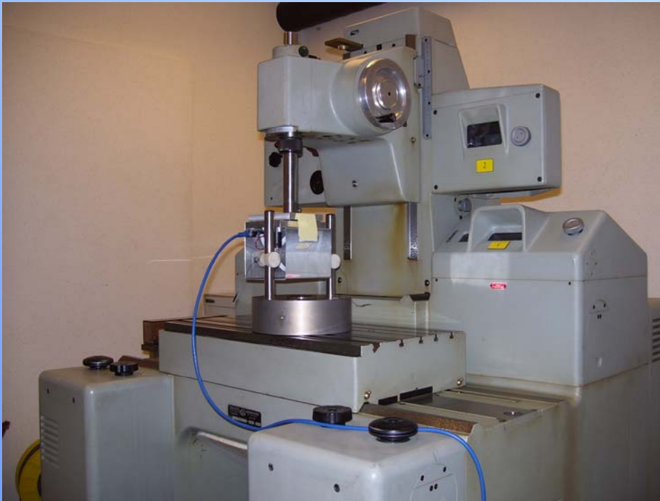
The Trioptic 3D measuring machine from SIP (Geneva). (equipped with laser interferometer for measuring the translations)
