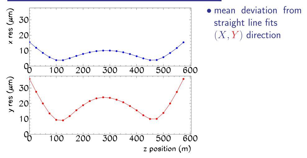
• statistical component of error budget well below specification:  $\sigma_x = 500 \mu m$ ,  $\sigma_y = 200 \mu m$
