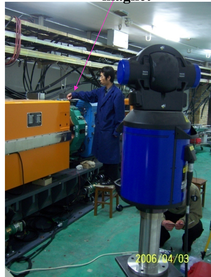
Fig. using the laser tracker to adjust the magnet
