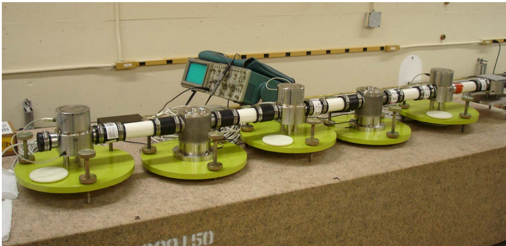
The first two prototypes of ultrasonic HLS sensor at SLAC, September 2005.
