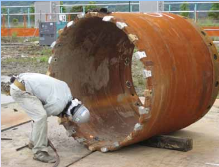
Pillar Casing Bit with Diamond Blades
