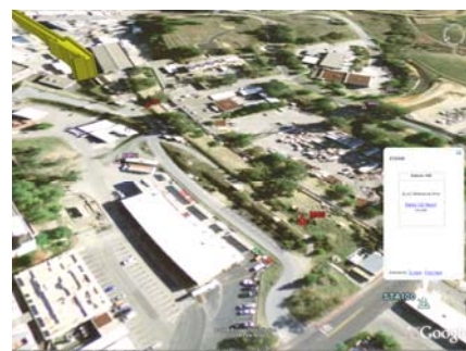
A screen-shot of the 3D model in Google Earth focuses on the the Beam Transport Hall (BTH). Spatially the tunnel is shown in its correct position relative to the geo-referenced aerial photos of SLAC found in Google Earth. By selecting a placemark (information point), the relevant Sharepoint surveying data is displayed.
