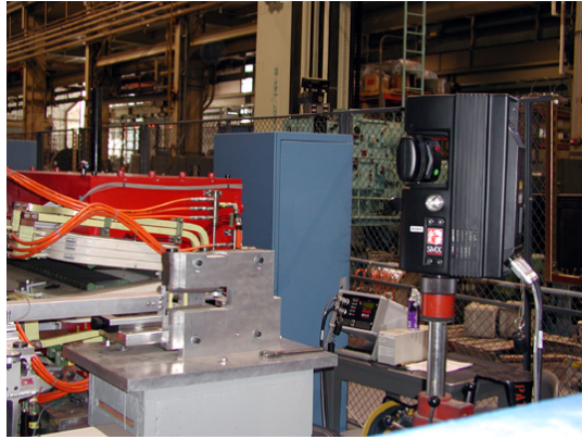
Fig. 2 Gradient Dipole Magnet (left) and Laser Tracker with Garage (foreground)
