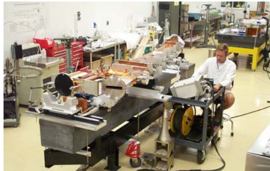
Fig. 6 Fiducialization of Vacuum Chamber
