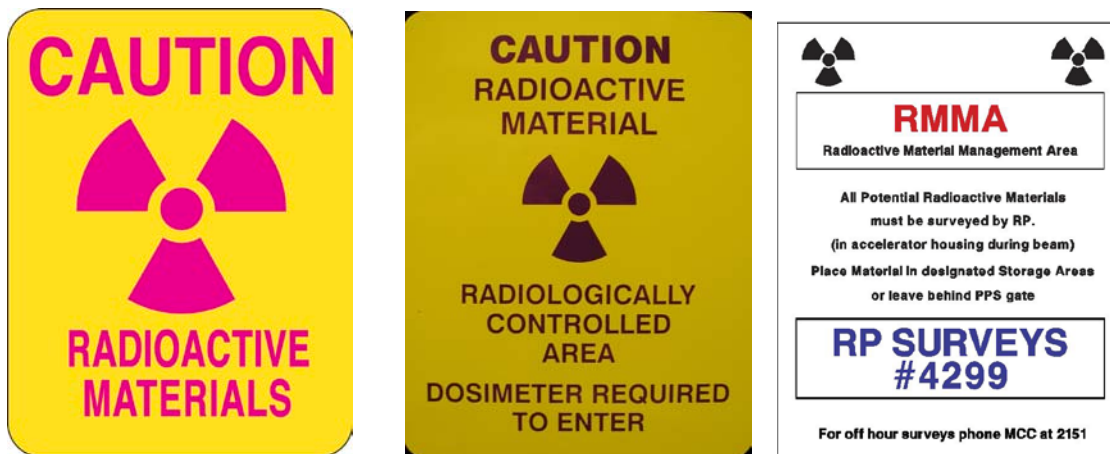
Figure 6-5 Radioactive Material Area Posting Types
