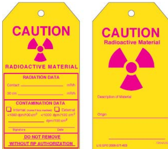
Figure 6-4 A Yellow and Magenta Tag Indicates the Item Is Radioactive
