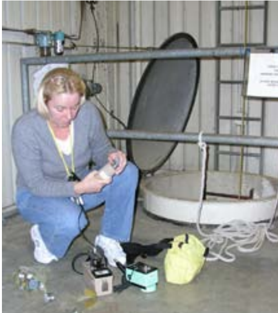
Figure 6-6 RPFO Technician Surveying Material for Radioactivity
