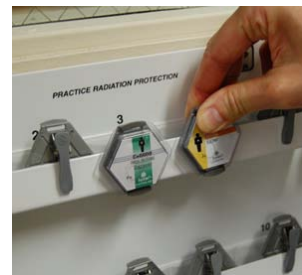
Dosimeter Storage Rack
