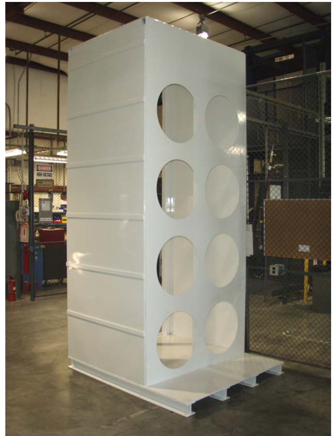
Figure 9. External Casing for the 150kW Test Load.
